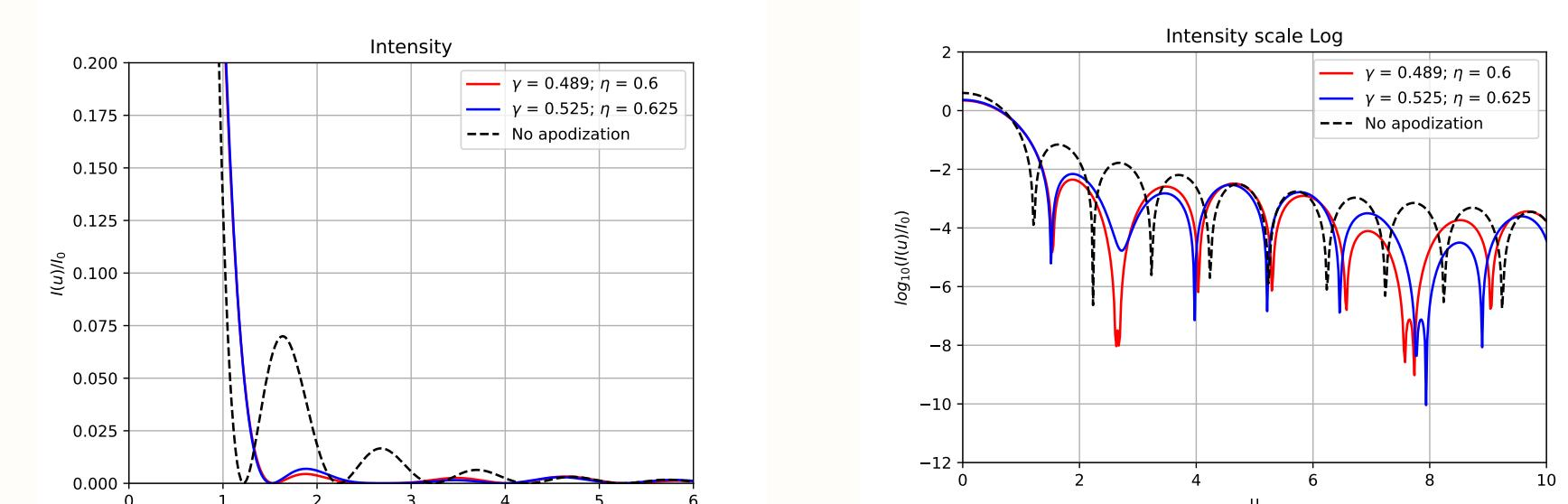
Figure 2: Left: Radial sections of the normalized PSF intensities. Right: in Log.
