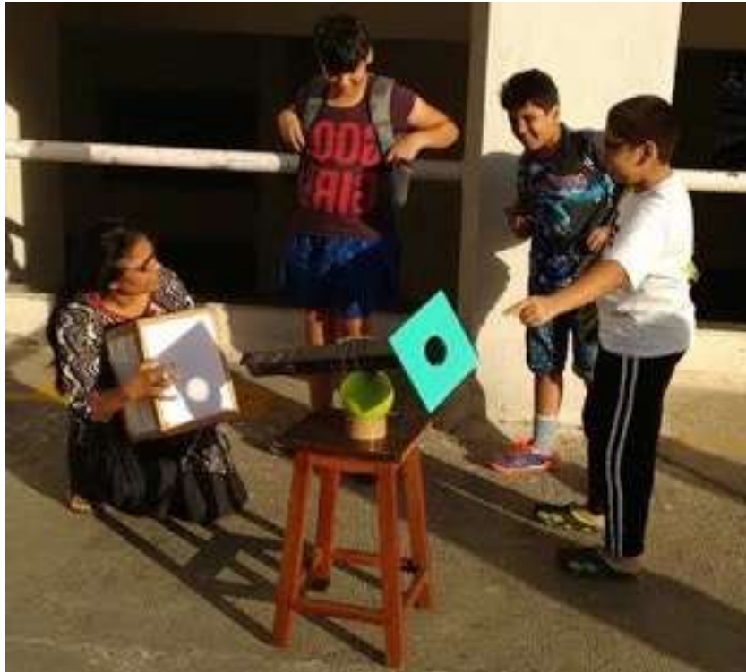
Projecting an image of the Sun onto a screen. The green cardboard blocks direct sunlight from the screen, increasing the contrast. Image courtesy: Navnirmiti Learning Foundation.
